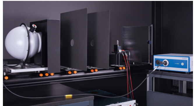
Fig. 1: Measurement setup for the calibration of a spectrometer with integrating sphere to irradiance with a reference lamp.
