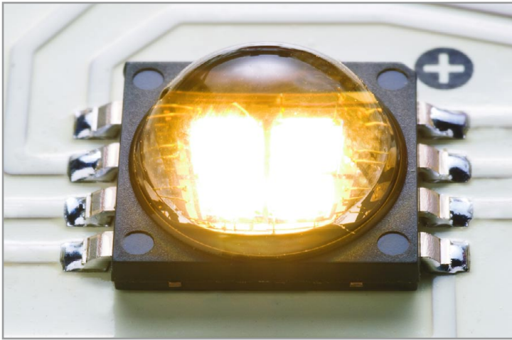
The multi-chip XLamp MC-E retains the same 7mm x 9mm footprint as Cree's existing XLamp XR family LEDs
