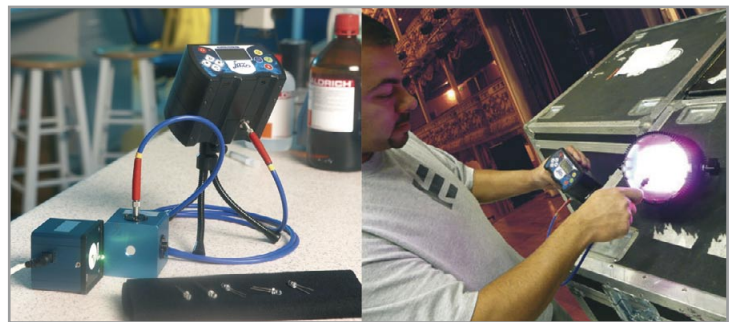
Figure 6: Portable spectrometer measuring single LEDs (left) that will be used for entertainment light fixtures as the one shown at a concert hall on the right photograph
