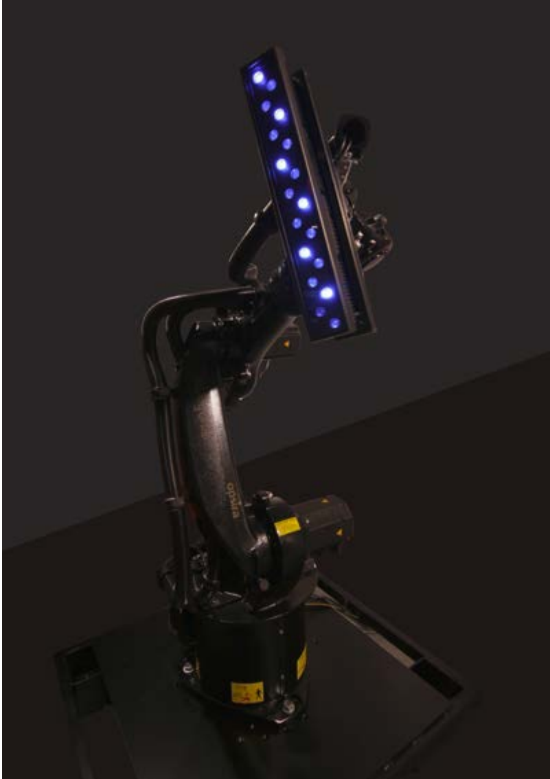
Figure 1: For LM-79 tests, luminous intensity distribution of luminaires is determined with goniophotometers
