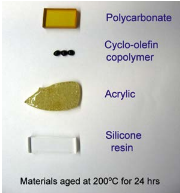
Figure 3: Comparative heat aging of polycarbonate, cyclo-olefin copolymer, acrylic and silicone resins after 24 hours at 200°C
