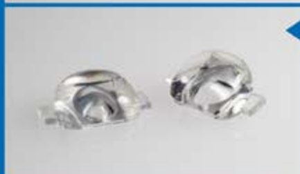
TUNNEL LL01CR-DL90120L02 L26 / W15.8 / H 9.15 FWHM 90° x 120° For Cree XPE
