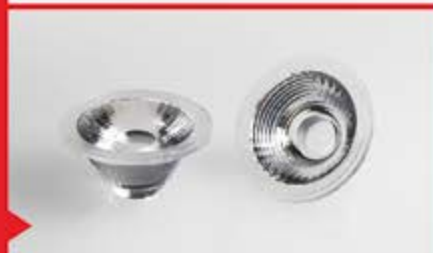
LL01ZZ-AHZxxL02 D x H (mm) 22.2x10.3 FWHM 24° 38° For Cree XML EZW
