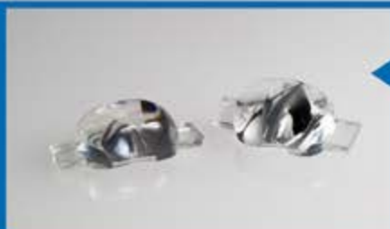
TUNNEL LL01CR-DL70130L02 L26 / W12.8 / H 8.65 FWHM 70° x130° For Cree XPE
