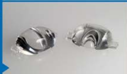
LL01LU-AGV80150L02 L32 / W18.5 / H9.5 FWHM 80° x 150° For Cree XM-L / MKR Luxeon M -Asymmetrical
