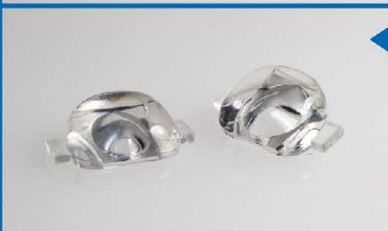
TUNNEL LL01CR-DL90120L02 L26 / W15.8 / H 9.15 FWHM 90° x 120° For Cree XPE
