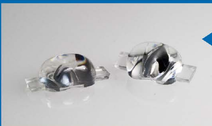
TUNNEL LL01CR-DL70130L02 L26 / W12.8 / H 8.65 FWHM 70° x130° For Cree XPE
