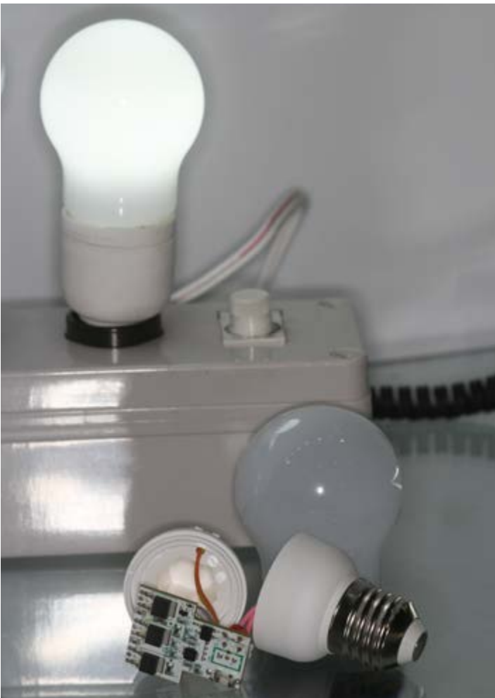
Figure 9: Rich Wall Technology's replacement bulb has the exact same dimensions as an Edison bulb
