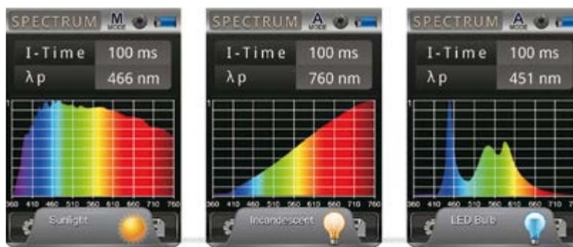
Figure 3: The measured spectrum characterizes the type and qualification of a light source
