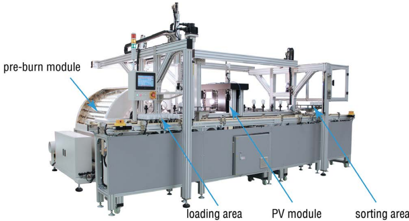
Figure 12: Automatic production test line with pre-burn module
