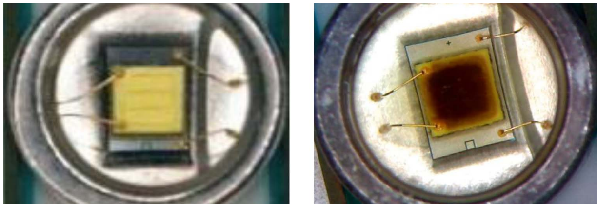
Figure 2: Examples of normal (left) and VOC degraded (right) LEDs
