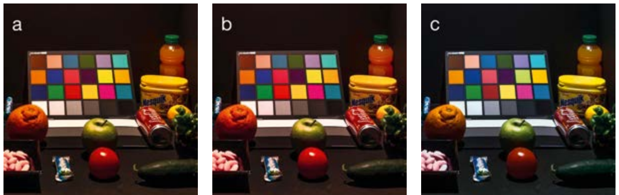
Figure 2: (a) Incandescent simulation, (b) neodymium simulation, and (c) cool white FL simulation
