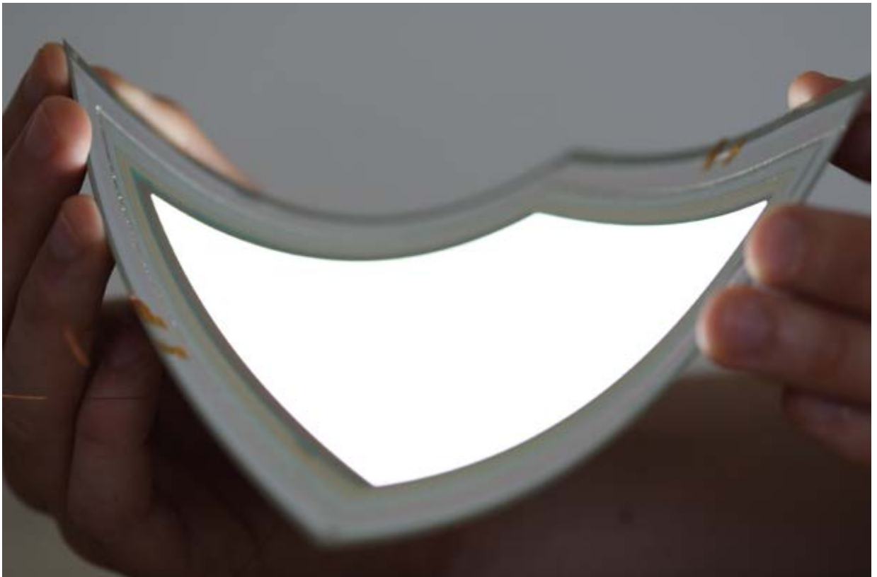
Figure 18: One of the major trends and success factors that Prof. Kido addressed in his speech were flexible white OLEDs (credits: Holst Centre), as well as transparent, color tunable and large area OLEDs
