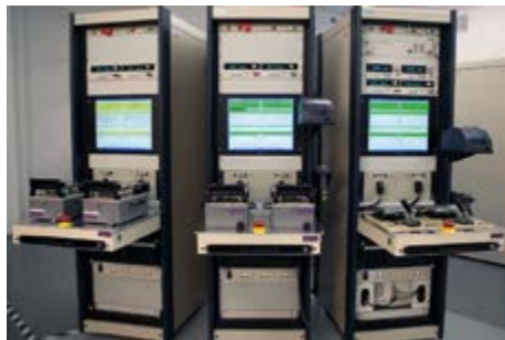
ASE's test system can be used to test LED luminaries with up to 300 VRMS (750VA maximum) or 425 VDC (575 W maximum)
