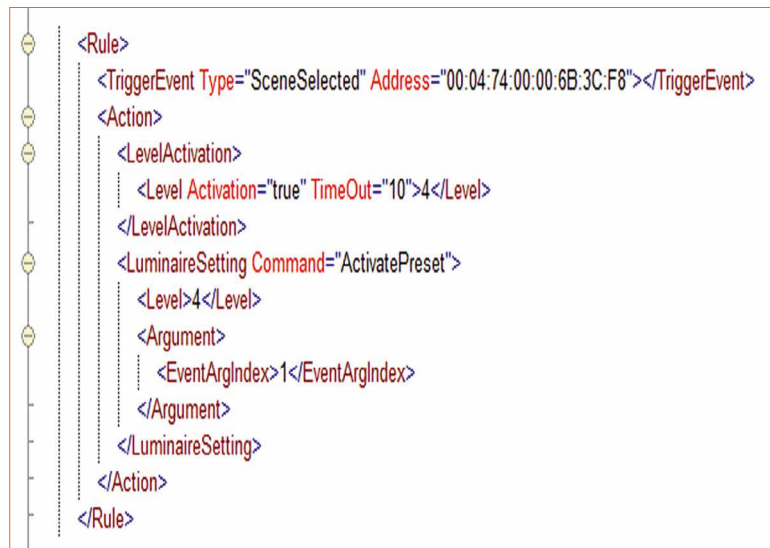
Figure 9: XML presentation of a rule - The event "SceneSelected" is generated by a 6 button panel. The event comes with one parameter representing the pressed button number. This parameter is passed to the "LuminaireSetting" command "ActivatePreset". So the shown rule will activate a preset depending on which button has been pressed
