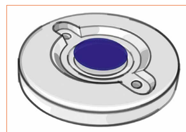
Figure 2: A Zhaga Book 3 LED module. The Ideal Light-Emitting Surface (LES) is indicated as blue disc. Note that the disc is elevated above the actual LED module's physical features in this example
