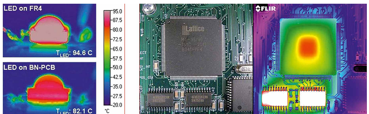
Figure 1: The images below show the thermal impact of LEDs and of other devices such as processors
