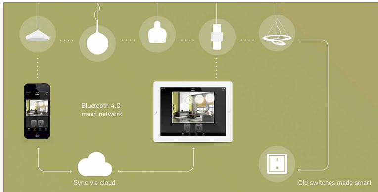
Figure 2: A typical Bluetooth 4.0 lighting mesh network configuration
