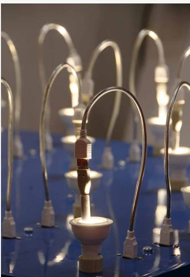
TUV SUD demo lifetime test setup for MR16/GU10 lamps at LpS 2015
