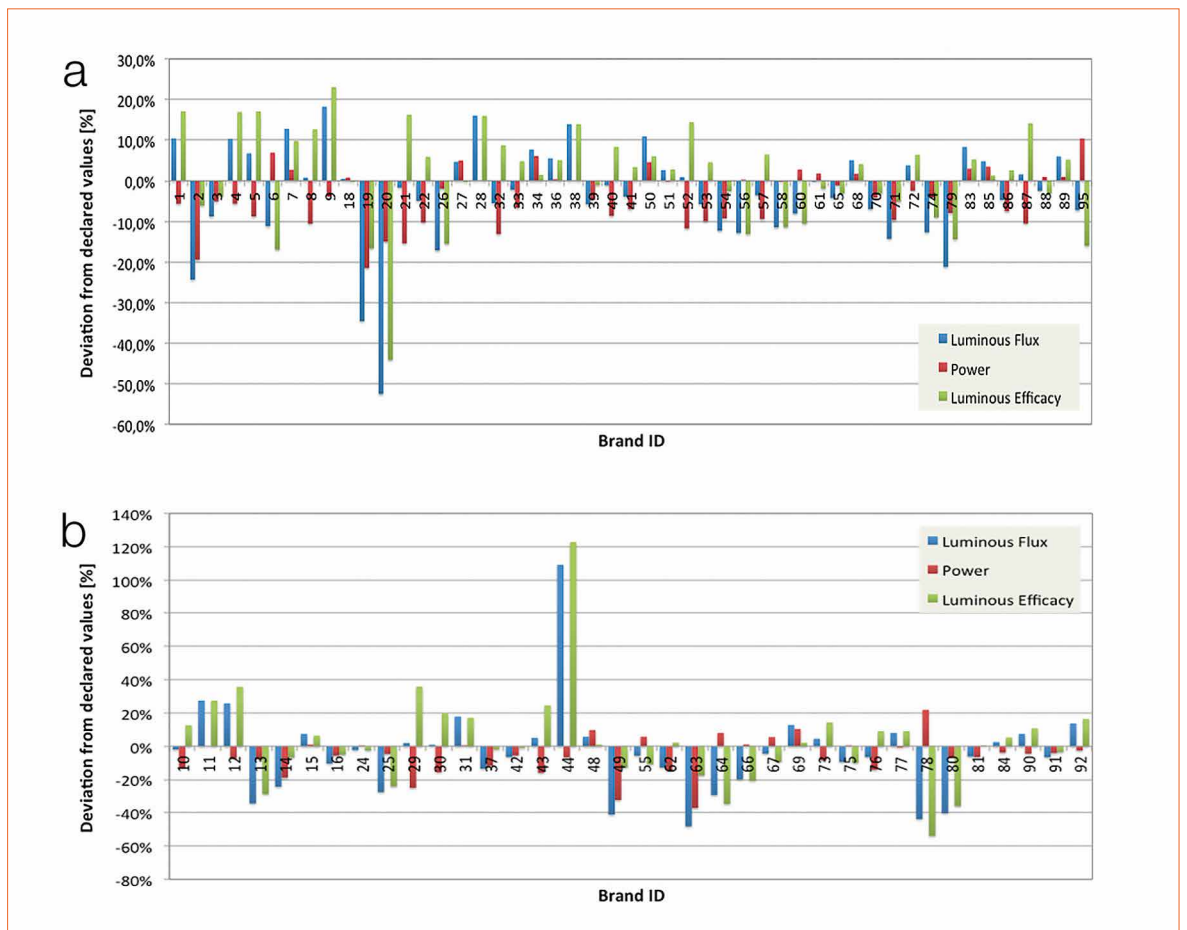
Figures 3a&b: (a) Observed deviations between declared and measured for input power, luminous flux and luminous efficacy values for LED bulbs (b) Observed deviations between declared and measured for input power, luminous flux and luminous efficacy values for LED spots
