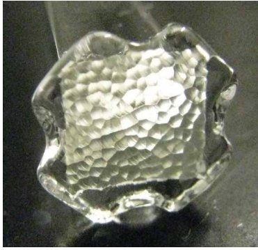
Figure 7: S3 structure on a complex light guide exit surface
