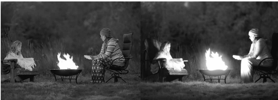
Figure 2: The pictures demonstrate the differences in absorption and reflection of visible (VIS) radiation (left) and near infrared (NIR) radiation (right). - For comparison reasons both images are held in gray scales
