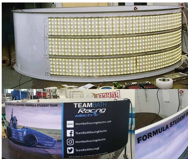
Figure 4: Flexible, R2R overmoulded RGB LED foil was used to build dynamic, large area, and curved advertisement display
