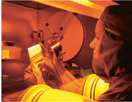
Flexible photovoltaic elements, manufactured at the pilot plant of the Fraunhofer IAP
