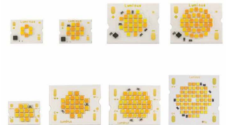
An on-board IC on Luminus' Warm Dimming Modules (top) enables standard drivers and dimmers to deliver halogen-like illumination from 3000 to 1800 K with a typical CRI of 92 or 97 while CCT Tunable Modules (bottom) deliver a wider individual tuning range
