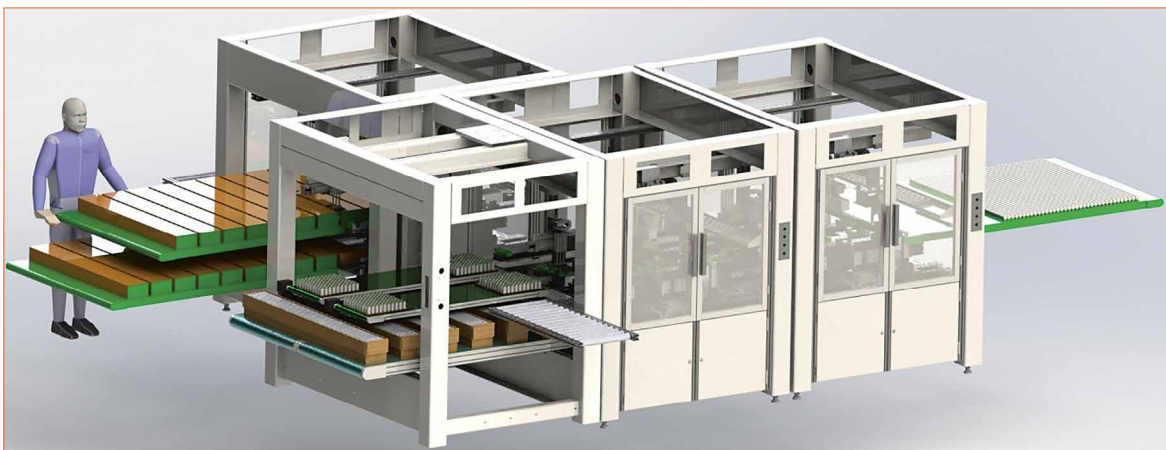
Figure 2: Simpler example of the microfactory, just using the loading, assembly and laser marking+ unloading modules
