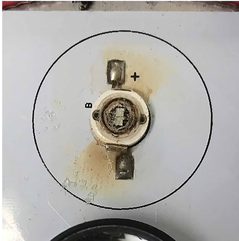
Figure 4: Example of an LED destroyed by heat trapped within the lens
