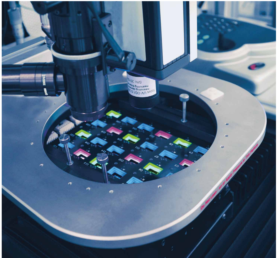
Probe station with patterned OLEDs in the clean room of Fraunhofer FEP (Credits: ©Fraunhofer FEP)
