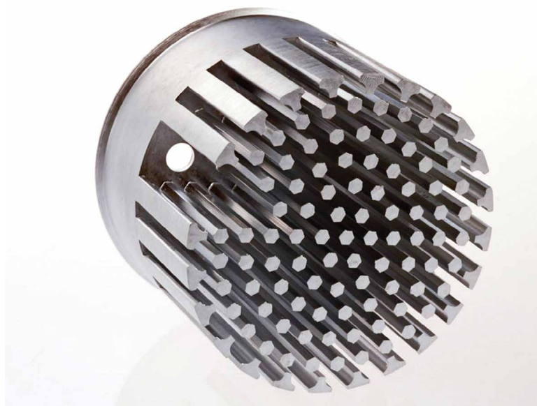
Figure 2: Cold forged aluminum heat sinks offer better thermal conductivity than die cast products
