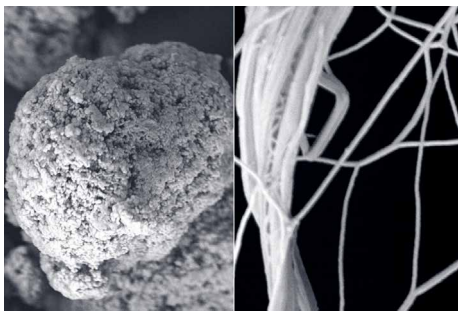
By mixing polymer powder in solution to generate a film that they then stretched, MIT researchers have changed polyethylene's microstructure, from spaghetti-like clumps of molecular chains (left), to straighter strands (right), allowing heat to conduct through the polymer, better than most metals
