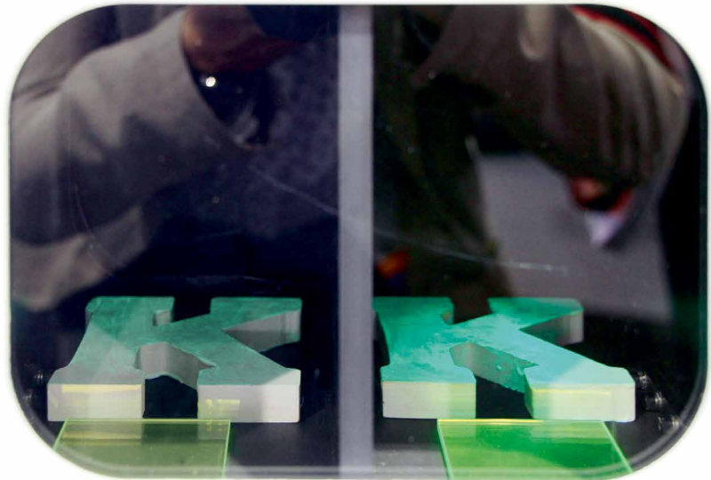
▲ Using UV-fluorescent materials, Kopp Glass demonstrated the benefits of UV-transmissive glass optics for UV LEDs
