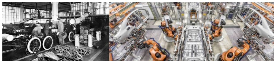
Figure 2: Manual line production (left), individual mass production by robotics (right) [1,9].
