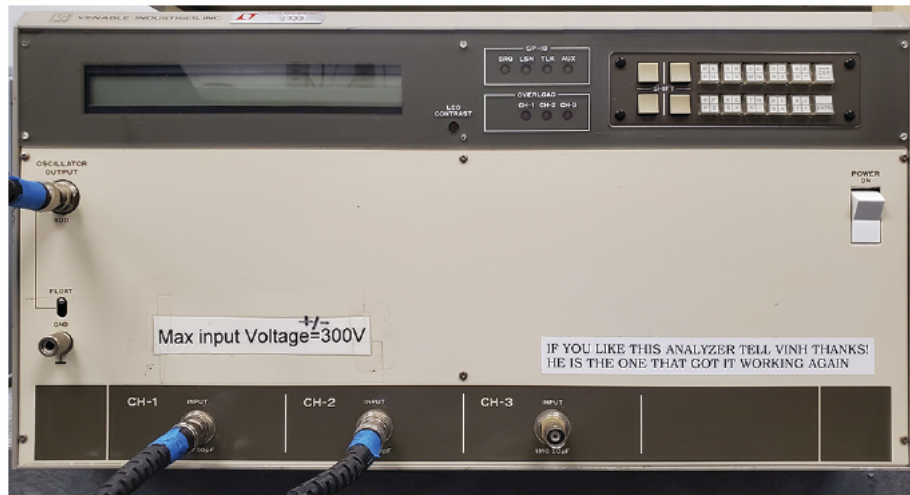
Figure 6: Venable System Model 5060A vintage network analyzer used for high-side floating noise injection and measurement of LED drivers.
