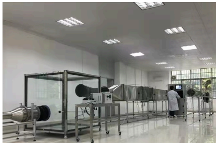
Figure 3: Testing of a 3,000 LPM air disinfectant at the Guang Zhou Institute of Microbiology, achieving a 99.96% single pass kill rate against aerosolized Staphylococcus aureus .
