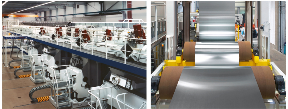
Figure 3: Roll-to-roll coating line with in-vacuum deposited large area coatings for high quality and cost-efficient metal reflectors.
