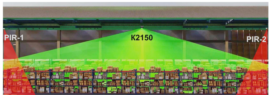
Figure 2: Sensitivity areas of PIR sensors in the beginning and in the end of the warehouse aisle (highlighted in red) and a sensitivity area of a radar sensor (highlighted in green).
