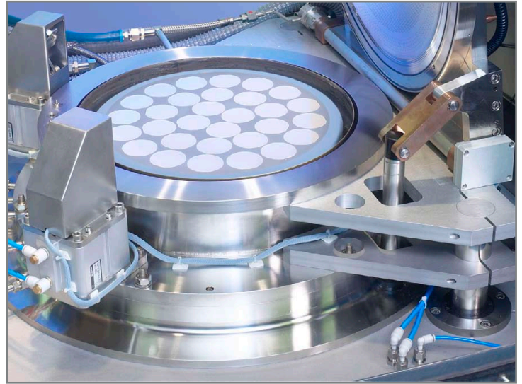
Figure 3: CRIUS® CCS reactor in 30x2" configuration for blue, green or white LEDs
