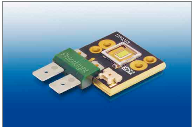
Figure 3: Construction of PhlatLight CBT-120 package. The actual PhlatLight chip is directly bonded to a copper heat spreader, which also includes a thermistor, connector and protective window.
