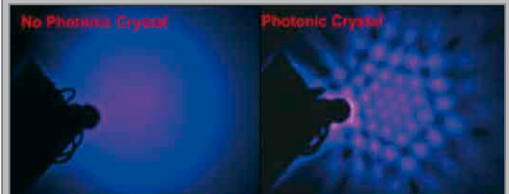
The photonic-crystal LEDs strongly modified far-field pattern shows a triangular symmetry due to the extraction of waveguided modes and showed a 50% increase in efficiency compared to the controls
