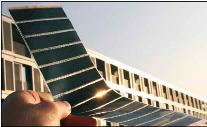
Figure 2: Most recent technology - CIGS flexible module from Flisom AG
