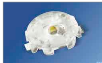
Figure 13: OSRAM Golden Dragon ARGUS® for a round beam
