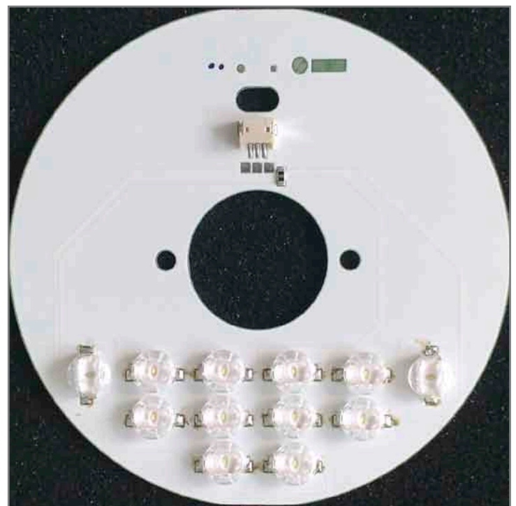
Figure 3: High-performance MCPCB LED board
