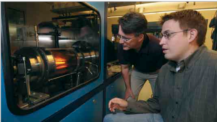
Timothy D. Sands (left) and a graduate student operate a "reactor" in work, which deposits gallium nitride on silicon at temperatures of about 1,000 degrees Celsius.
