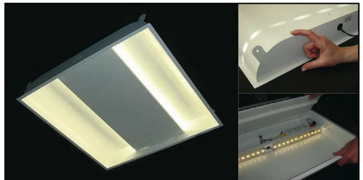
Axiom AX2424 LED fixture features indirect reflected lighting. The Low profile fixture drops in and easily replaces existing fluorescent fixtures. Mounting brackets are provided for securing the fixture as required. Axiom AXLE8 modules are easily replaceable with twist of the vinyl knurled mounting screw.
