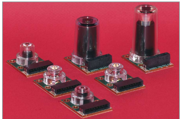
Figure 1: LumiBright LE line of light engines for commercial applications and incorporating high efficiency primary optics, photosensor, and thermistor on a high thermal conductivity metal core PCB in one package.
