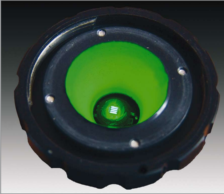
Figure 5: Cone adapter to 'stretch' the integrating sphere isolates assembled LEDs for test.
