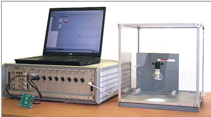
Figure 3: The T3Ster thermal tester was used to physically test the MR16 retrofit LED lamp application.
