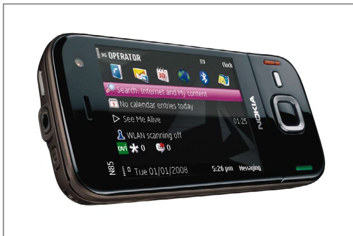
Figure 1: For mobile phone displays, OLEDs have several advantages over other solutions, but they are expensive and have - with about 10,000 hours - a shorter life time than their anorganic relatives.
