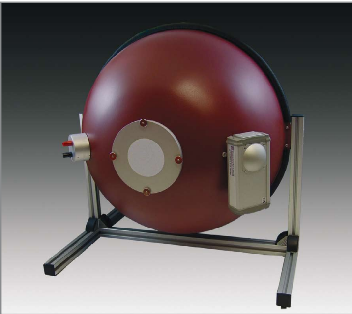
Figure 6: Large diameter integrating sphere with large measurement port enables the measurement of the total flux and averaged color data of LED arrays.
