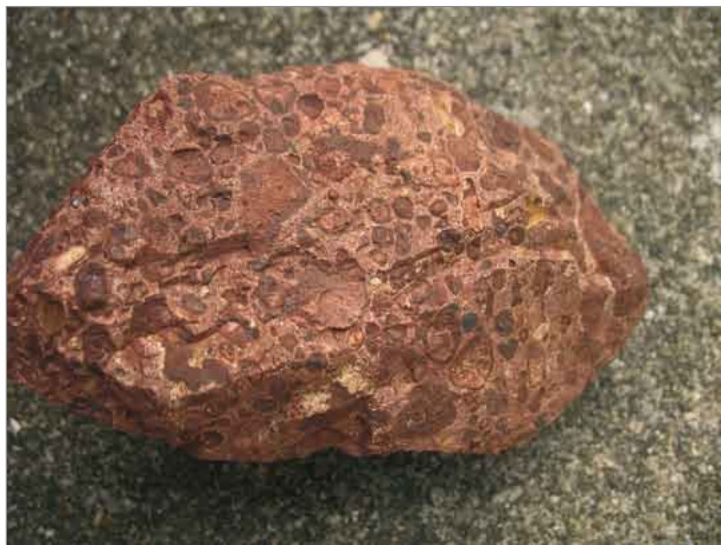
Figure 1: Bauxite raw material: The basis for the production of aluminum and ceramic (Credits: Geological collection, University of Tübingen, Dr. Udo Neumann).
