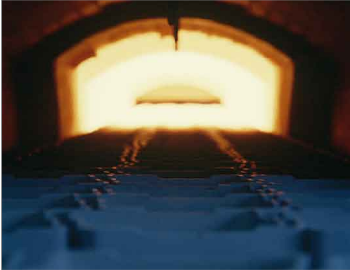
Figure 3: Sintering - Formed ceramic parts undergo heat treatment below the melting temperature; alumina Al 2 O 3 , e.g. at 1300-1600 °C (air). Sintering uses the most energy of all process steps in the production of ceramic, yet the amount of CO 2 released is only half the amount released in aluminum production.
