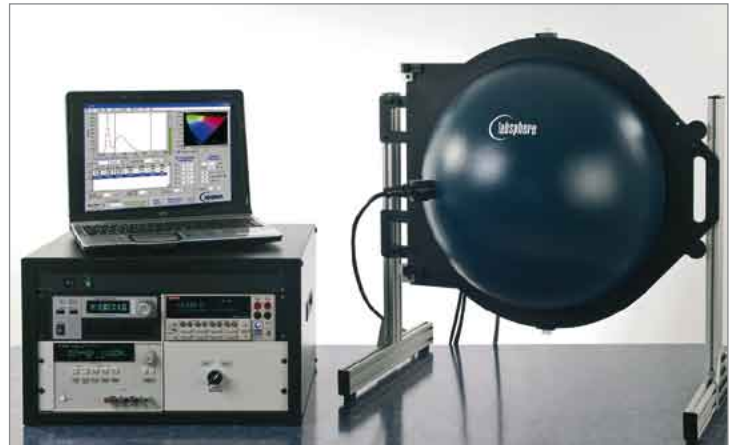
Labsphere's TOCS system conforms to IESNA LM-79 and LM-80 recommendations for LED characterization.
