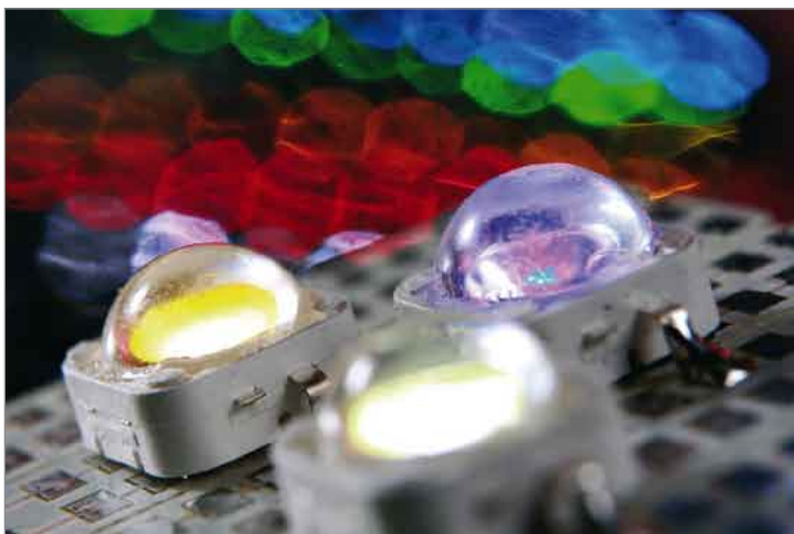
Figure 1: An LED package with a low thermal resistance, like the TitanBrite High Power LED package, is mandatory for manufacturing durable, efficient high quality solid state lighting products.
