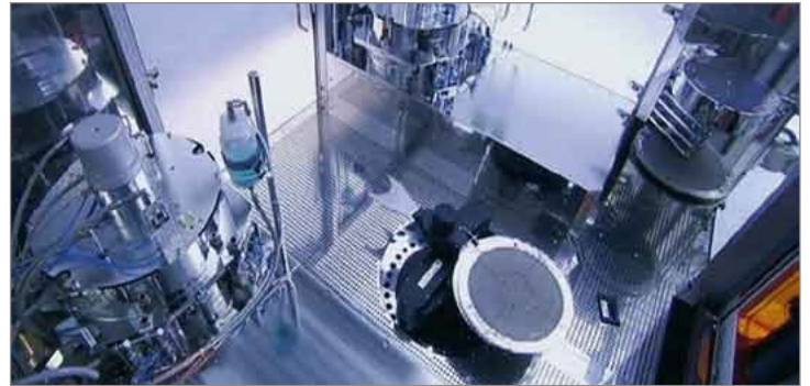
The EVG®560 HBL is a dedicated, fully automated wafer bonding system for High-Brightness LED manufacturing.
