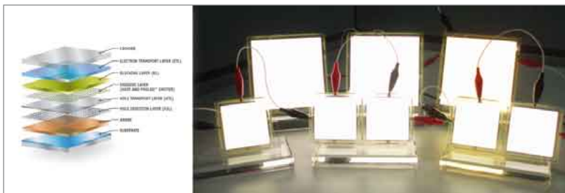
Figure 4: New improved OLED structures allow higher luminosity, recently up to 3,000 cd/m 2
