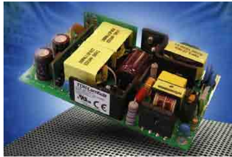
TDK-Lambda's ZPSA100 series power supplies are compact with up to 90% efficiency
