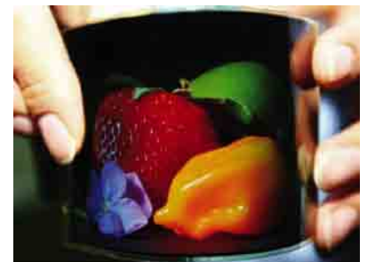
Figure 5: New AMOLED displays have a narrow bending radius
