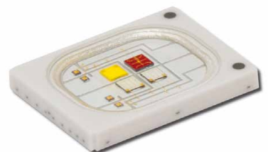
The Z-Power LED Z6 is a RGBW LED with a total power consumption of 4 W
