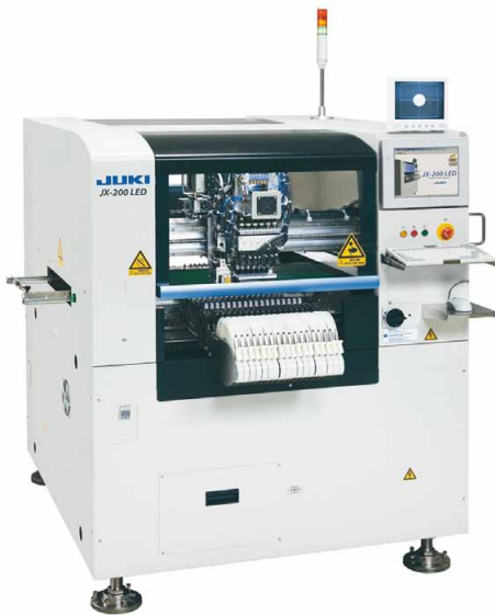
Juki JX-200LED is designed especially for the LED assembly market
