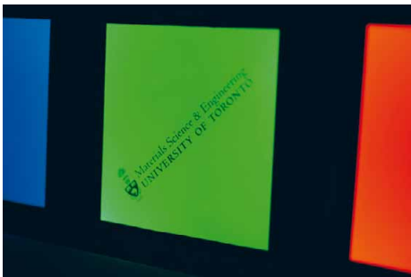
Red, green and blue CI-ITO-OLEDs from the University of Toronto Material Science and Engineering Institute
