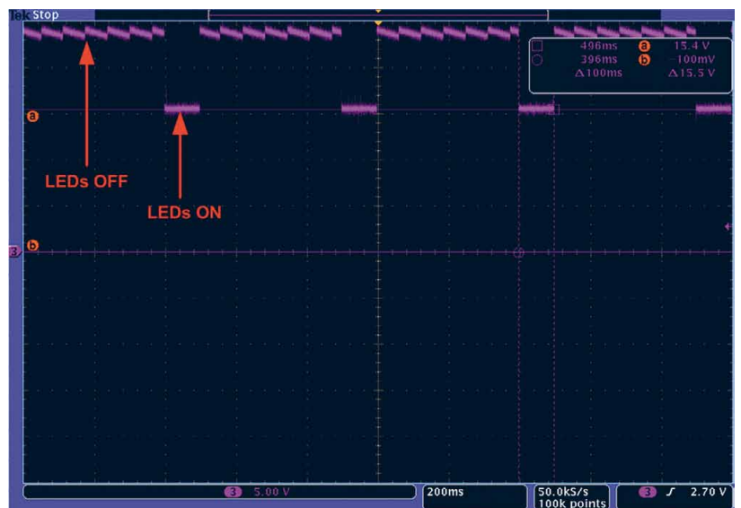
Figure 6: Scope plot of boost converter's LED drive
