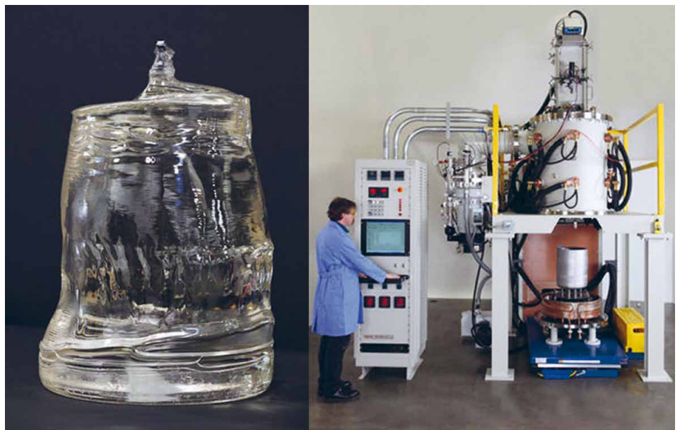
Sapphire substrate (left) for LEDs, grown with Thermal Technology's K1 crystal grower
