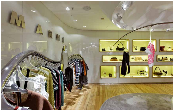
Sybarite chose to use MEGAMAN's LED PAR30 15W light sources to recreate the original lighting scheme's warmth and drama. A mock-up test in the store assured that the required light levels were being obtained...
