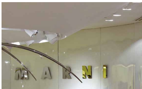
Sybarite chose to use MEGAMAN's LED PAR30 15W light sources to recreate the original lighting scheme's warmth and drama. A mock-up test in the store assured that the required light levels were being obtained...
