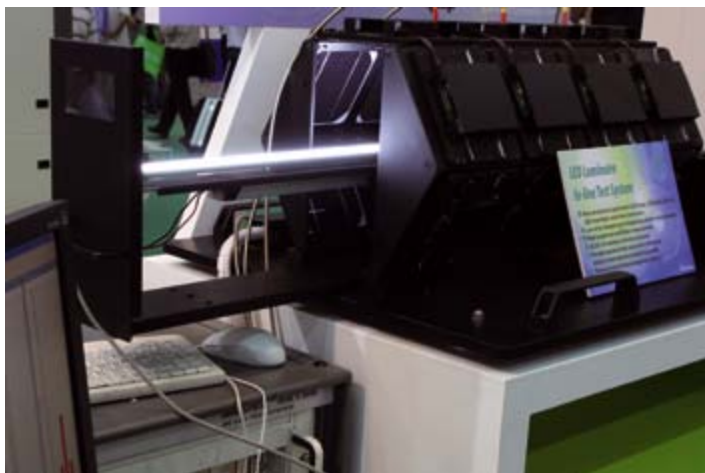
Figure 3: Chroma's LED Luminaire In-Line Test System uses PV cells to measure light distribution and intensity
