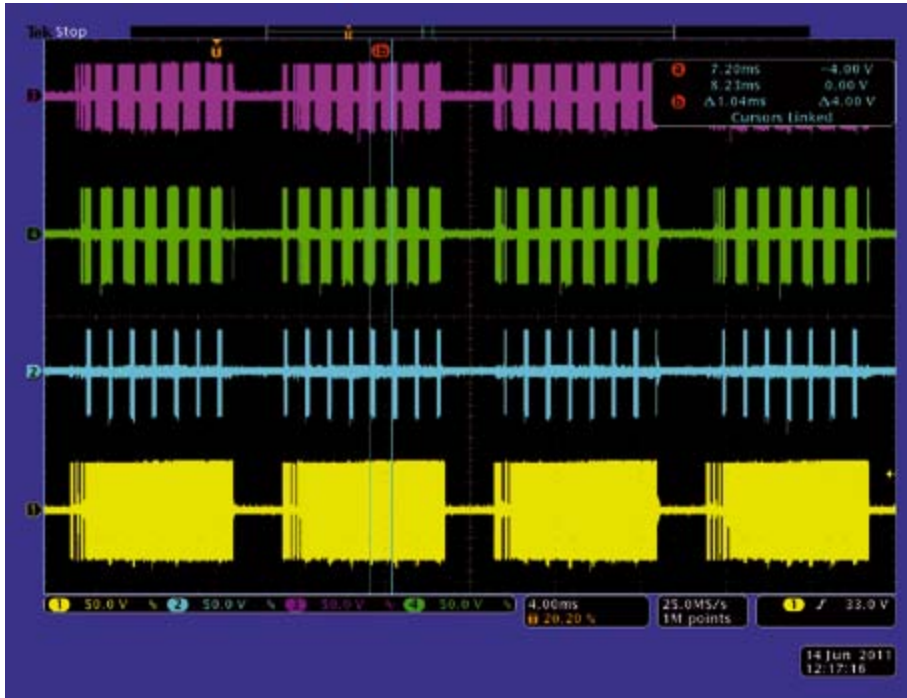
Figure 7: RGBW with different dim-level each channel
