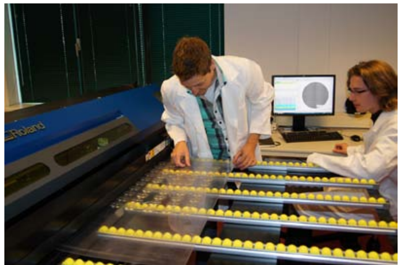
Figure 1: Making optical products with print-optical technology on a modified Roland printer. The yellow rollers are for guiding the substrate
