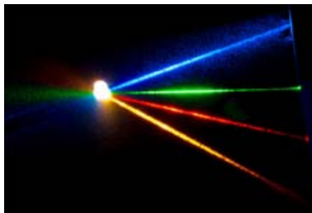
Four laser beams — yellow, blue, green and red — converge to produce a pleasantly warm white light (Photo by Randy Montoya)
