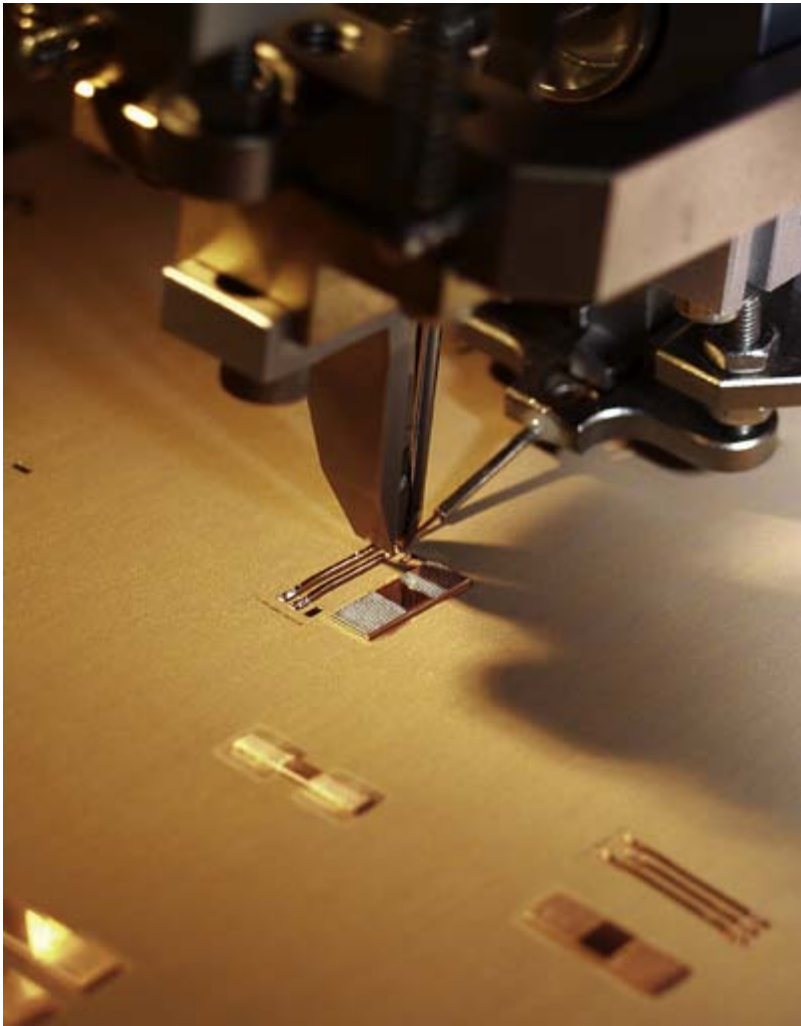
Figure 2: Exterior copper components within the type of wires or profiles are deposited directly onto the base copper by means of ultrasonic welding
