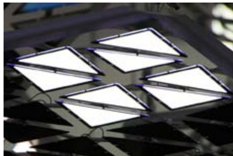
OLEDs, like all organic electronics, are very sensitive to water vapor and oxygen, hence need to be well protected
