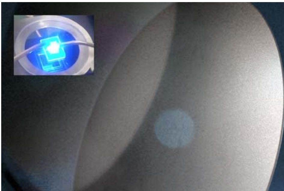
NGK's GaN wafers promise improved internal quantum efficiency - small image shows LED element under light emitting test (Substrate size: 1cm square, Element size: 0.3 mm square, Injection current: approx. 200 mA, Center wavelength: 450 nm)
