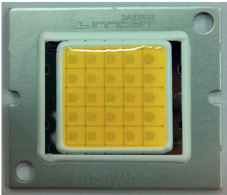
Daewon Innost's Glaxum™ LED Array, Chip-On Board module performs at 0.41°C/Watt
