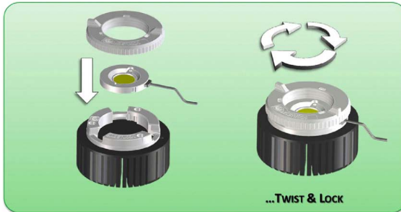
Figure 4: When the module is positioned inside the holder, the rotation of the ring gives the required pressure to the module against the heat sink and fixes the module in the correct position
