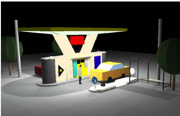
Figure 3 & 4: "AutoMat", self-service gas station-simulation in Dialux (left). "AutoMat", illuminance level-simulation in Dialux - white equals 250 lx (right)
