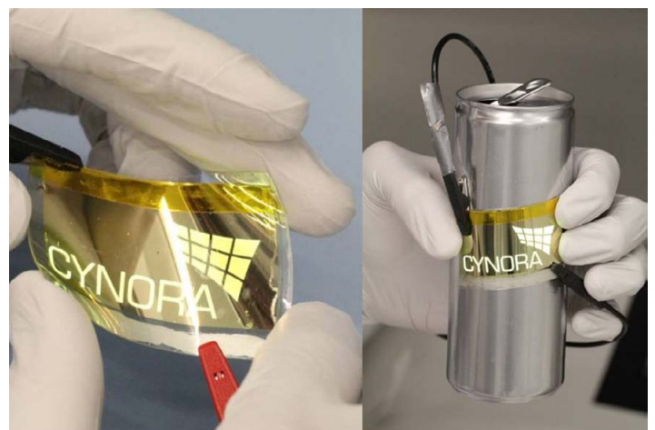
A thin film replaces rigid glass to produce a flexible OLED (left). Flexible OLEDs pave the way for intelligent packaging in the future (right)
