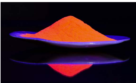
Intematix's new GAL phosphors, which are backed by U.S. patent No. 8,274,215, enable near-perfect color rendering up to 98 CRI
