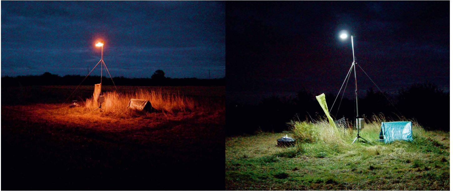
Figure 2: An increasing number of studies have examined differences between the ecological impacts of commercially available LEDs and existing street lighting technologies. Here, lighting rigs (L: high-pressure sodium; R: commercially-available LED) used in a study of impacts on nocturnal pollination by moths [13] are shown
