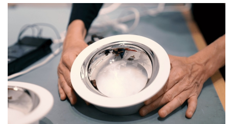
PHABULOU produces free-form micro-optical components. Image: Zumtobel Lighting GmbH.
