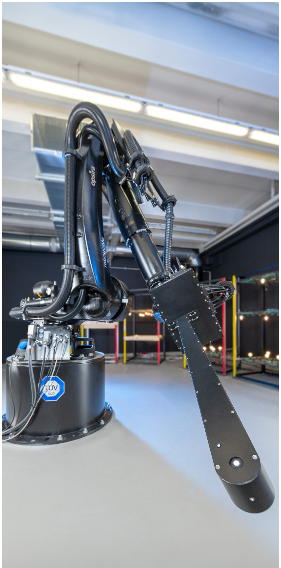
The robogoniometer at TÜV SÜD in Garching provides fully automatic 24/7 measurements of LED light output.
