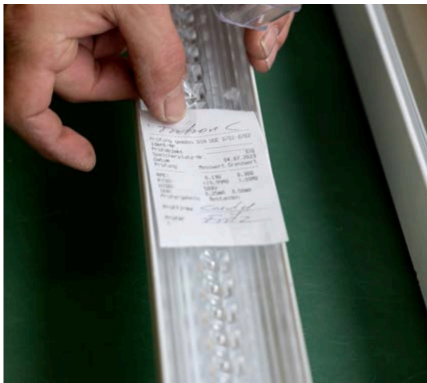
After testing the luminaires a test report is issued and the luminaires labelled.
