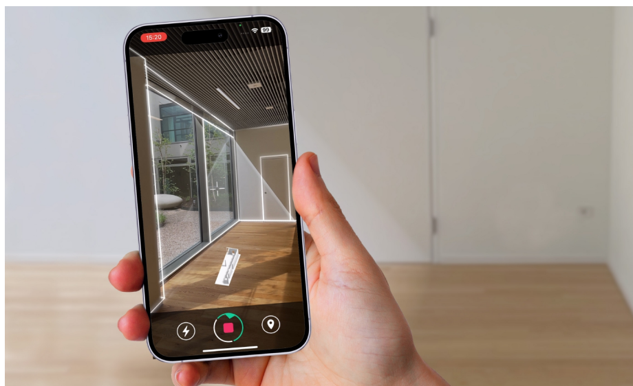
Figure 3: A 3D model is generated based on a smartphone's scan.
