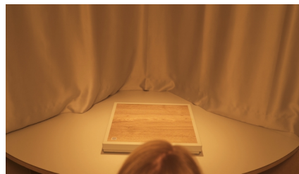
Figure 6: Frontal view of an evaluation station with the material samples centrally arranged in the table segment and the curtain elements located in the surrounding area to separate the evaluation booths.
