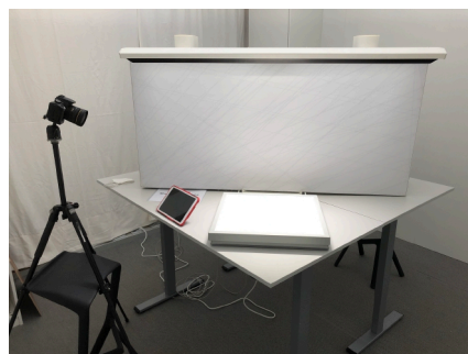
Figure 2: Frontal view of an evaluation station with the diagonally arranged lighting prototypes and the applied material positioning.
