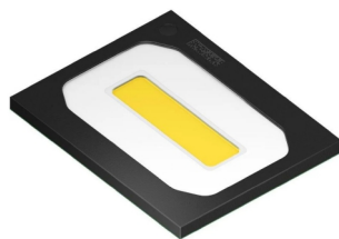
The EVIYOS® Shape, developed by ams OSRAM, is a disruptive LED technology featuring a monolithic chip with 25,600 micro-LEDs, each controllable with a 40 µm pixel pitch.
