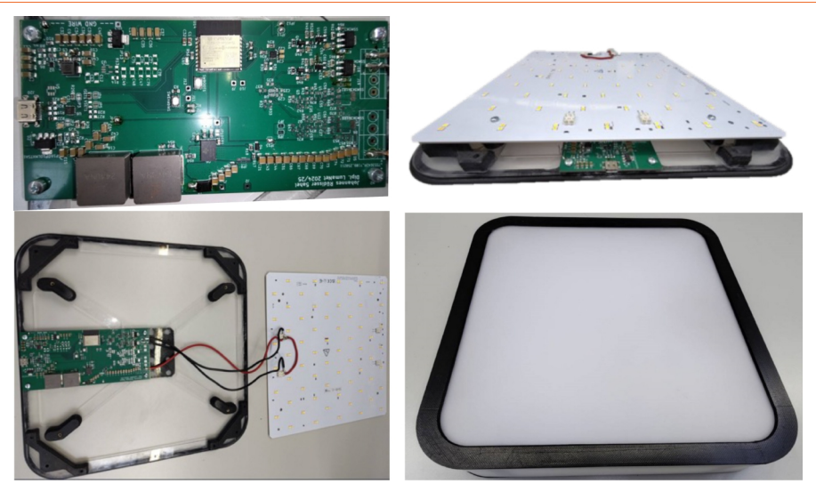
Figure 8: LED driver sample (top left). LED driver with USB-C connector mounted under LED panel (top right). LED driver and LED panel (bottom left). Luminaire prototype (bottom right). ©HTLR/SZK
