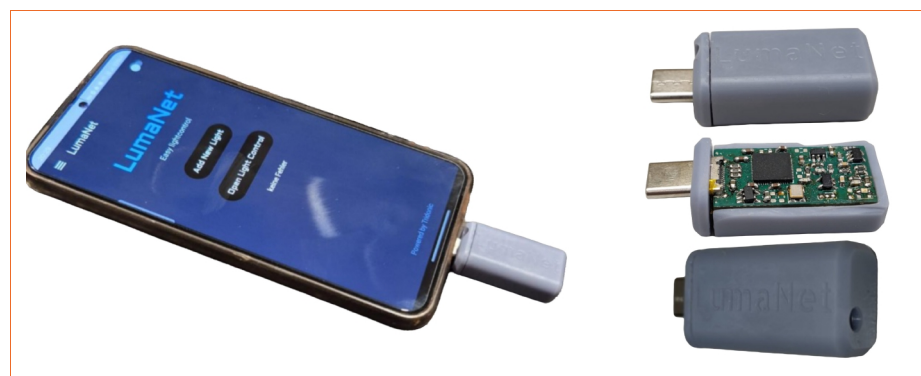
Figure 13: Smart phone with LumaNet app and mounted sensor (bottom). Sensor in enclosure (right top). Sensor controller HW (right middle). Optical Tunnel on rear side (right bottom). ©HTLR/SZK
