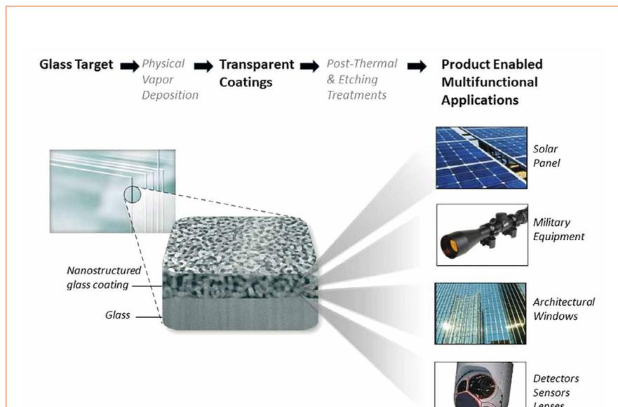
Schematic representation of the coated product and applications. The properties could also be useful in different lighting applications like outdoor lighting, street lighting or automobile headlights
