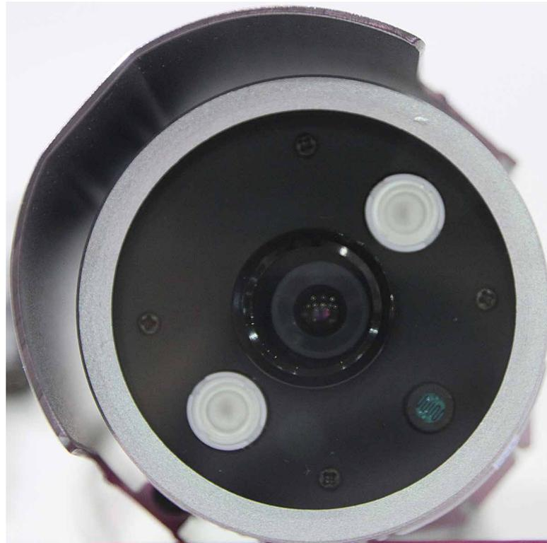
IR LEDs and UV LEDs have a number of very important applications in our daily lives. While IR LEDs are indispensable components of surveillance cameras, UV LEDs are used for the curing of plastics and other tasks
