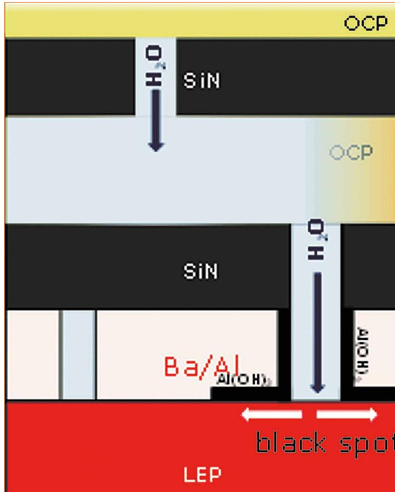
Figure 2: Pinhole-pinhole coupling leading to black spot growth in the device [2]
