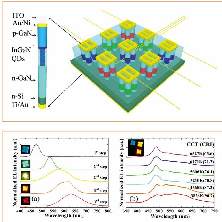
the backside of the Si substrate, respectively. In this study, the multi-color InGaN LED devices exhibit excellent current-voltage characteristics, including relatively low series resistance ( $\sim 20 \Omega$  or smaller).
