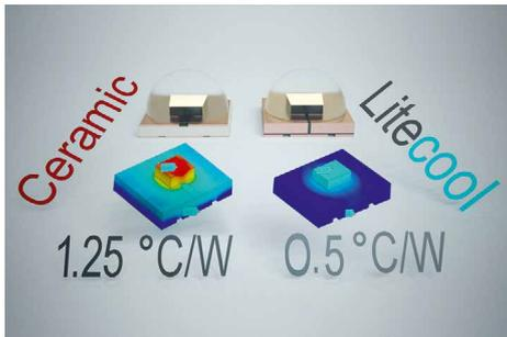
Litecool's new packaging concept significantly reduces the thermal resistance of LED packages by using a vertical dielectric
