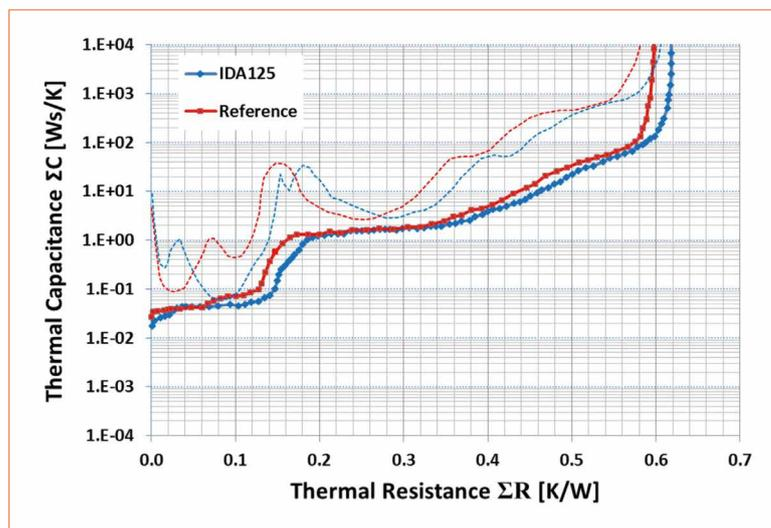
**Figure 3:** Thermal resistance comparisons as cumulative structure function for 75 W LED COB modules with IDA-125 and reference die attach products
