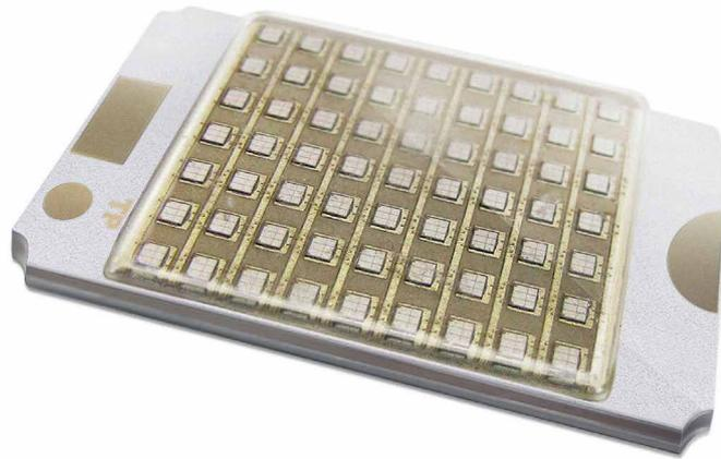
**Figure 2:** LED chip-on-board (COB) module (75 W) comprising 63 385 nm UV chips in a 7x9 configuration on an aluminum ceramic substrate utilized for thermal resistance testing of IDA-125 and a commercial reference product
