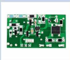
The ICL8201 is highly integrated, with the result that additional external components can be added with minimal effort. The control concept of the IC supports DC and AC input as well as high Power Factor Correction (PFC), high efficiency levels and reduced EMI design in Critical Conduction operation Mode without zero crossing detection winding.
