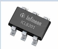
Infineon's new ICL8201 AC/DC buck controller with high power factor is tailored to cost-sensitive, non-dimmable LED retrofit applications. Its cascode structure current mode for non-isolated floating buck topologies provides constant current operation with low output ripple in a universal input voltage range.
