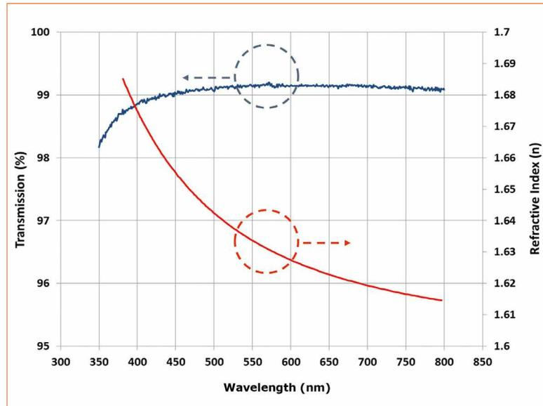
**Figure 1:** Transmission curve (blue) and refractive index dispersion curve (red) for a film of 70  $\mu\text{m}$  thickness formed the ILE-501 LED encapsulation product. ILE-501 part A & B were mixed in 1:1 ratio in a Thinky Planetary Vacuum Mixer for 2 minutes at 1400 rpm at 1 kPa. Glass slides were coated and the sample cured at 150°C for 60 min.
